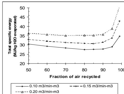
**Fig. 7.** Effect of the air flow rate on the specific energy consumption of the drying for a range of air flow rate and air fraction of air recycled. Conditions:  $M_{in}$  45 % dry basis,  $M_f$  0.5 % dry basis, bed thickness 0.25 m.
