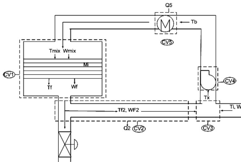
Fig. 1. A demonstration dryer used for STR 20 block rubber drying.
