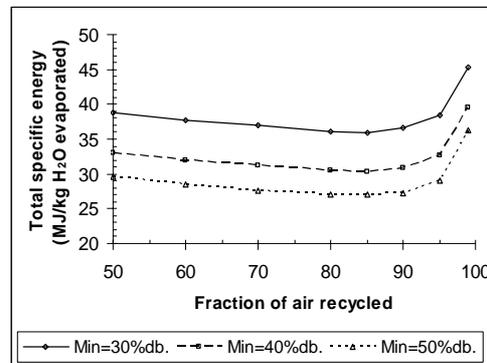
**Fig. 6.** Effect of initial moisture content of the rubber on the specific energy consumption of the drying for a range of initial moisture content and fraction of air recycled. Conditions: Bed thickness 0.25 m,  $M_f$  0.5 % dry basis, air flow 1.8 m/s.
