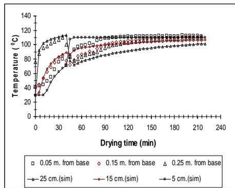
**Fig. 2.** Evolution of rubber temperatures according to drying time from experimental and simulated results. Conditions: Drying at 130°C for 40 min (air flow: top to bottom, 2.5 m/s) and followed by at 110°C for 180 min (air flow–bottom to top, 2.5 m/s),  $M_{in}$  46.65% dry basis.
