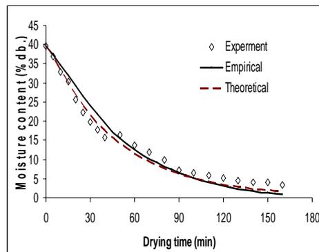
**Fig. 3.** Evolution of rubber moisture contents according to drying time from experimental and simulated results. Conditions: Drying at 130°C for 40 min (air flow: top to bottom, 2.5 m/s) and followed by at 110°C for 120 min (air flow – bottom to top, 2.5 m/s),  $M_{in}$  39.61% dry basis.
