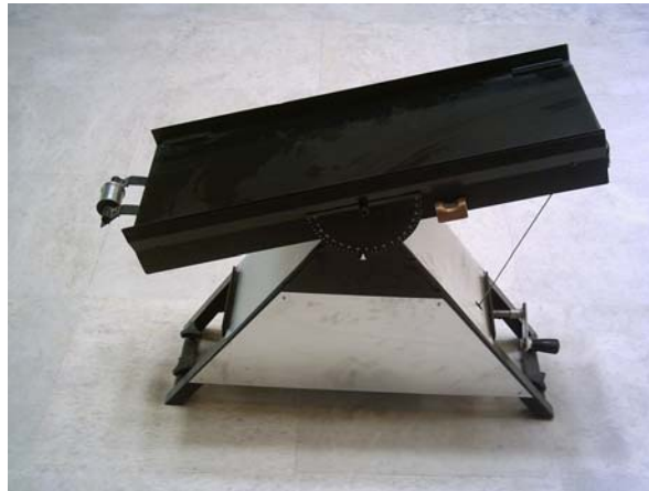
Fig. 1. Apparatus to determine emptying angle of repose
