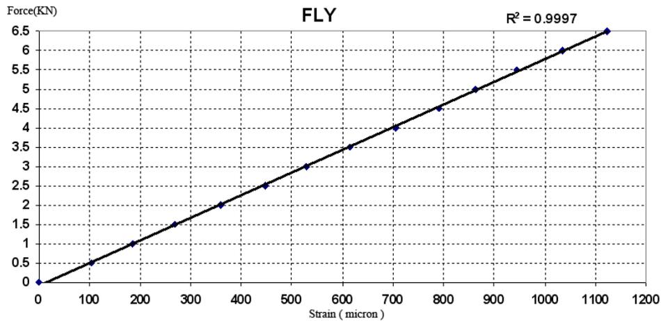
**Fig. 5.** Calibration curve of left arm.
