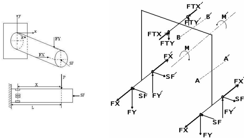
Fig. 3. Force diagram (A) and Force components on the elastic element (B).
