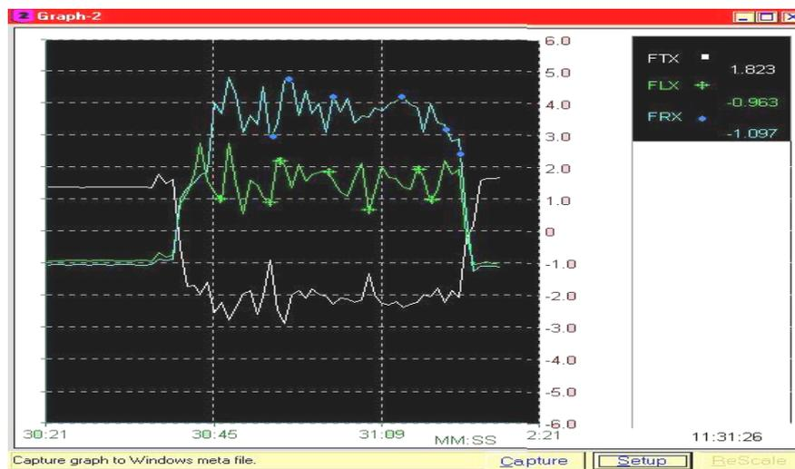
**Fig. 8.** Force diagrams of individual arms: right arm (upper curve), left arm (intermediate curve), and upper link arm (lower curve).
