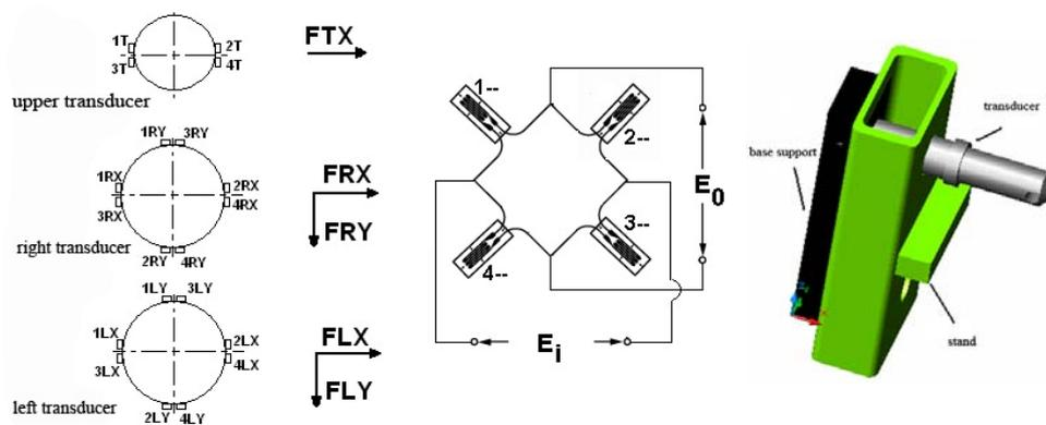
**Fig. 2.** Interface member along with transducer and arrangement of the applied strain gauges.
