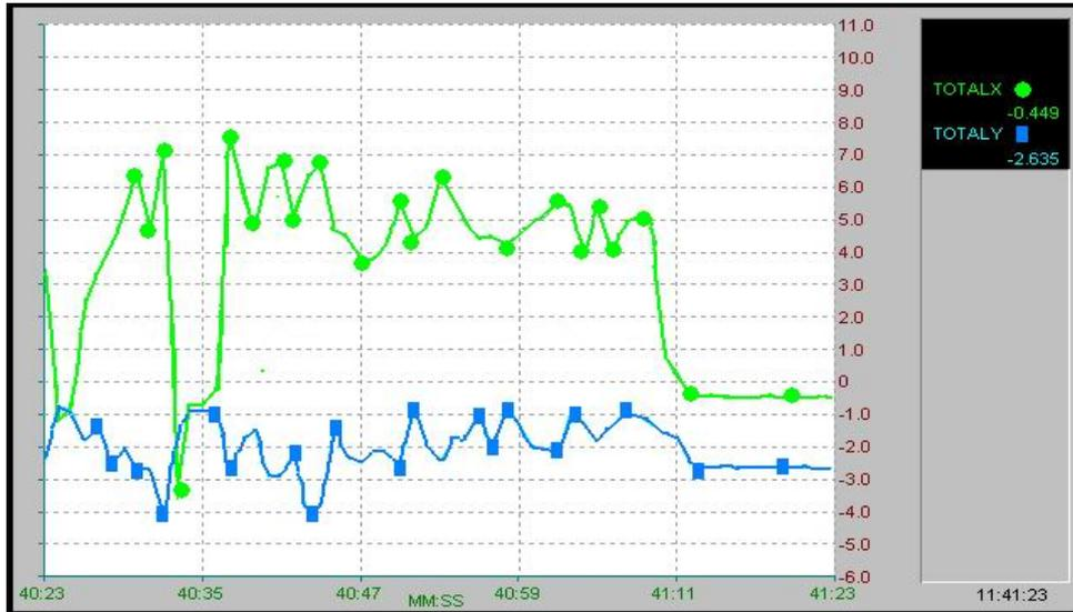
**Fig. 7.** Aggregate of horizontal force (upper curve) and vertical force (lower curve) of the tested dynamometer obtained in field test.
