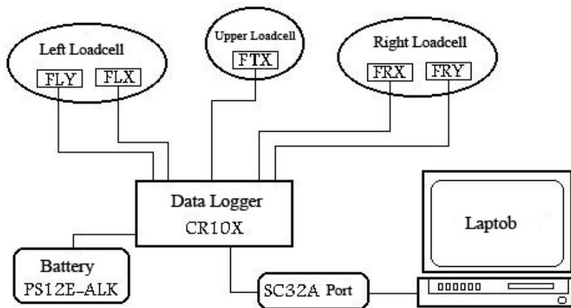
Fig. 4. Schematic illustration of all system.
