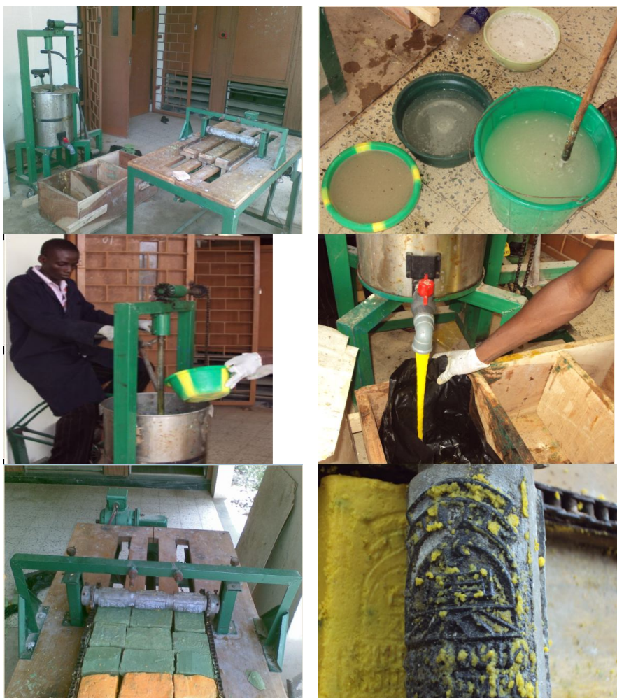
Fig. 2. Soap Making, Cutting and Stamping Processes
