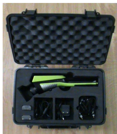
Fig. 2. ULIRVision TI160 thermal imaging camera
