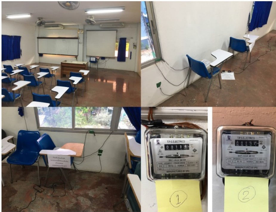
Fig. 8. Recording temperature and electricity consumption saving from PSA in sample classroom.
