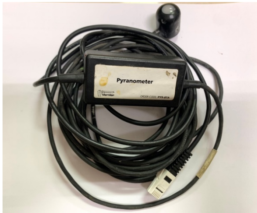
Fig. 5. Pyranometer for solar radiation.
