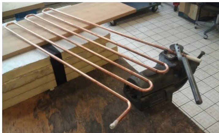
Fig. 6. Bending of a copper tube using hand bending machine.
