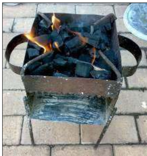
Fig. 2. A photograph of the traditional metal Mozambican charcoal stove.
