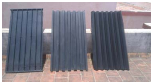
Fig. 2. Three different types of absorber plates (flat plate, square pulse and v-grooved).
