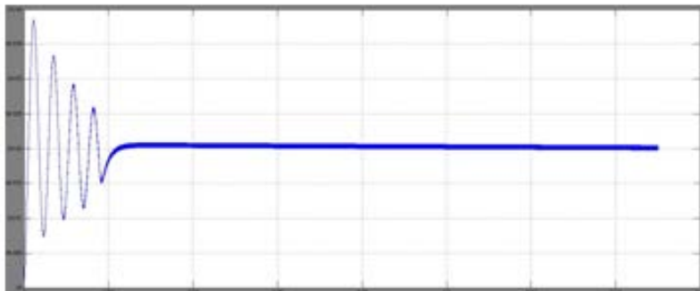
Fig. 17. Interleaved converter output with P and O MPPT at constant illumination.
