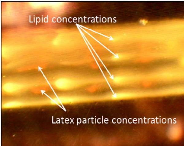
**Fig.7:** A nominal 1175  $\mu\text{m}$  embossed device filled with a mixture of 3  $\mu\text{m}$  latex beads and milk, with no flow. Nodal spacings in 2 dimensions are clearly seen.
