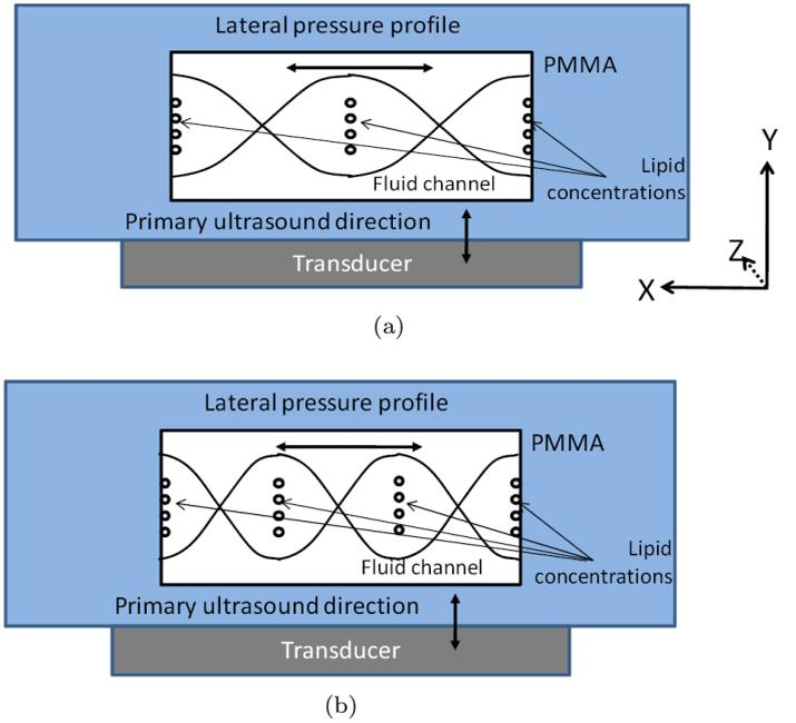
**Fig. 1:** Generation of lateral pressure profile within a) a 1 wavelength device, and b) a 1.5 wavelength device, orthogonal to primary acoustic direction, showing the position of lateral pressure nodes and antinodes.
