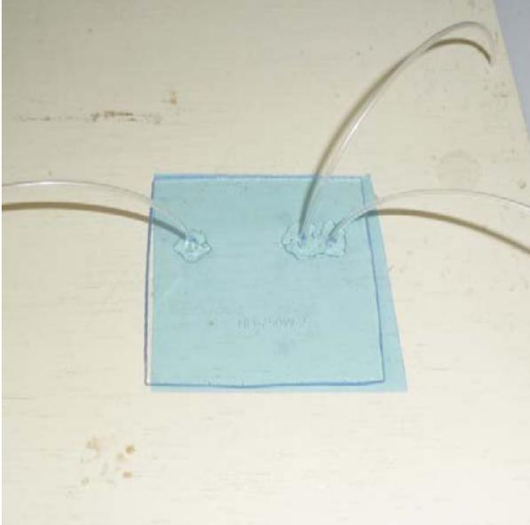
**Fig. 6::** The completed fluidic device, showing attached tubes for fluid access, bonded by epoxy adhesive (Araldite), prior to attachment of the ultrasonic transducer.
