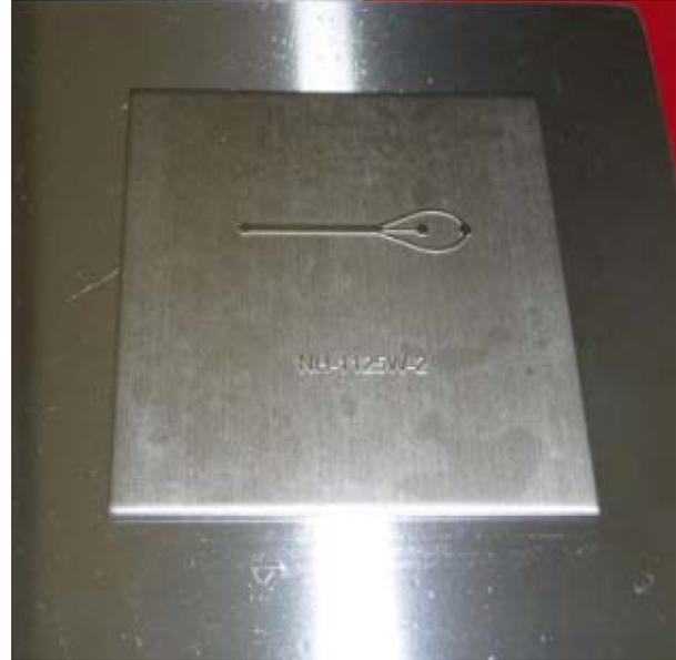
*Fig. 5:* Picture of an etched steel embossing mould.
