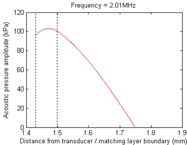
**Fig.2::** Modelled pressure profile through the multilayer structure. The air boundary is at 1.75 mm. The fluid layer is between the two dotted lines. The antinode is clearly seen between these lines.
