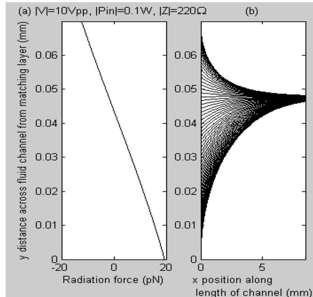
**Fig.3::** Dynamic modelling of lipid paths. The traces show the estimated trajectory of lipids as they progress down the first 8 mm of the fluid channel, at flow velocities of 5 mm/s.
