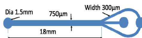
**Fig.4::** Planar separator design showing channel arrangement (inlet on left).
