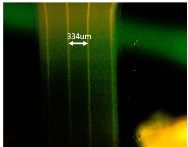
**Fig.10:** An embossed device, operating at 1.85 MHz showing tightly focussed lipid streams.
