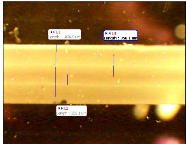
**Fig.9:** The milled device with latex particles and milk, with flow. The lines of concentrated material are more regular.
