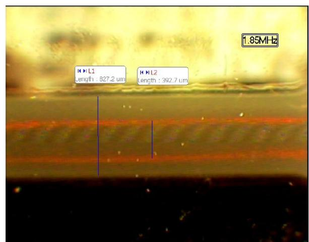
**Fig.11:** A 750  $\mu\text{m}$  device filled with 3  $\mu\text{m}$  latex beads, showing the formation of two bands of particles in the pressure nodes, at a frequency of 1.85 MHz.
