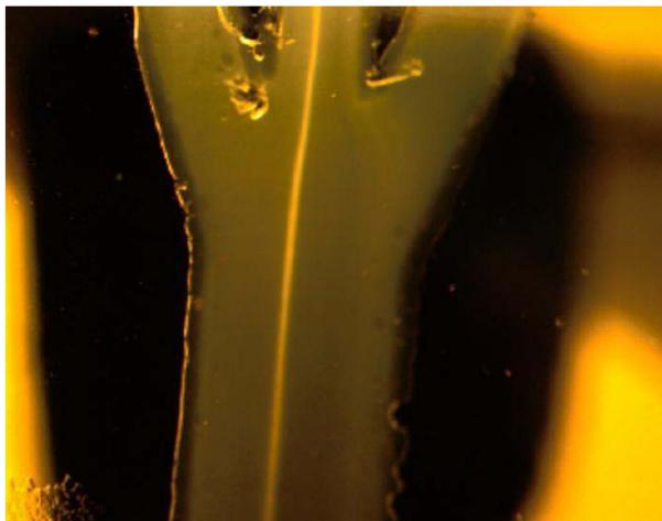
**Fig.12:** Outlet of 750  $\mu\text{m}$  channel showing concentration of lipids primarily concentrated into the centre laterally and moving through the centre outlet. Flow is from bottom to top.
