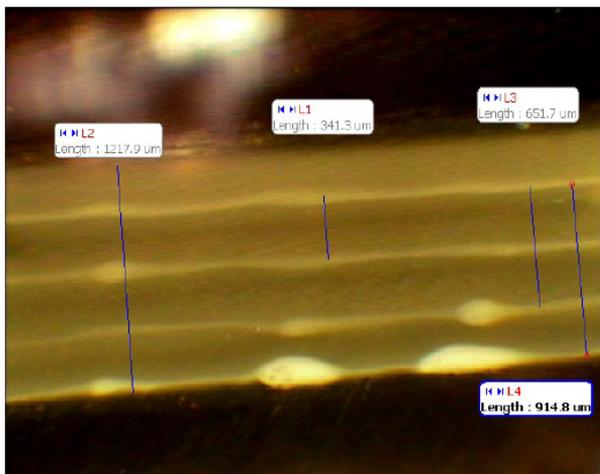
**Fig.8:** The same device as shown in figure 8 filled with milk and flow applied. Streams of lipids are clearly seen.
