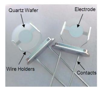
Fig.2: Piezoelectric Quartz Crystal Structures
