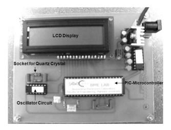
Fig.3: Oscillation Frequency Counting Device (Inhouse developing by Department of Biomedical Engineering, Faculty of Engineering, Mahidol University)
