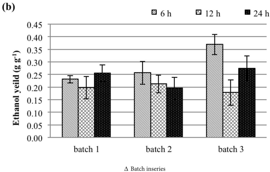
**Figure 7.** Ethanol productivity and ethanol yield at HRTs of 6, 12, and 24 hours under batch in series ( $p < 0.05$ ,  $N = 12$ )
