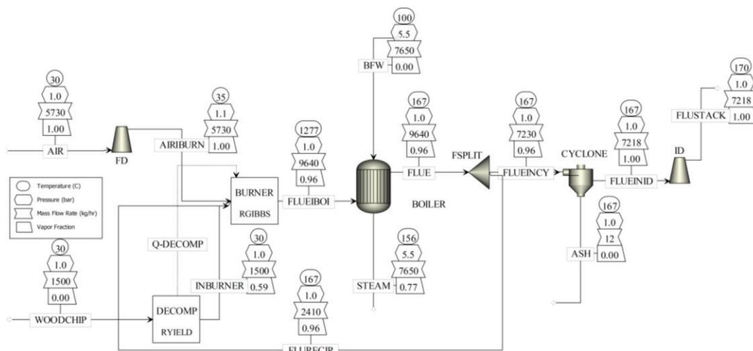
Figure 7. Process flow diagram under optimal conditions (Structure 2).
