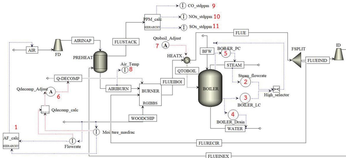
Figure 12. Process simulation with controllers by Aspen Dynamics
