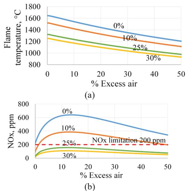
**Figure 5.** Effect of excess air at different amount of flue gas recirculation on (a) Flame temperature, (b) NO<sub>x</sub>, (c) CO, (d) SO<sub>x</sub>.
