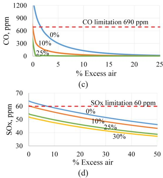
**Figure 5.** (cont.) Effect of excess air at different amount of flue gas recirculation on (a) Flame temperature, (b) NO<sub>x</sub>, (c) CO, (d) SO<sub>x</sub>.
