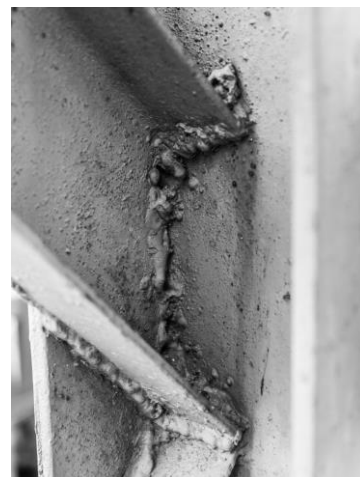
Fig. 7 Porosity and incomplete fusion of weld on a steel billboard
