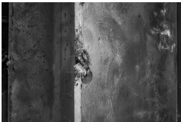
Fig. 8 Missing steel section melted by poor welding procedure
