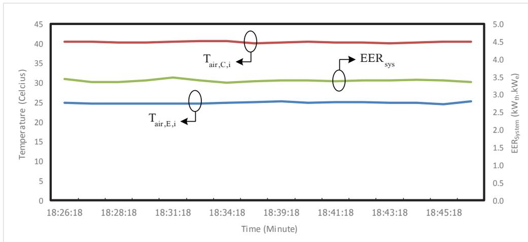
**Figure 11** The air temperature profile and  $EER_{sys}$  for R-32 air-conditioner at the air entering evaporator and condenser temperature around 25°C and 40°C with 10 m of piping tube.
