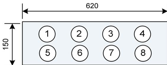
**Figure 6** The measuring positions of air velocity at the hood of the evaporator.
