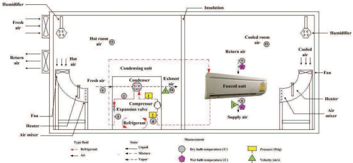
Figure 2 Measuring positions of the testing room for air-conditioner.
