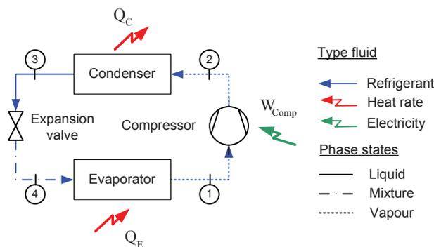
**Figure 1** A vapor compression heat pump [11].
