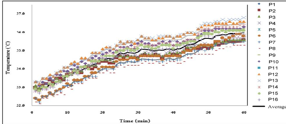
Figure 8 The air temperature profile of the condensing unit room.
