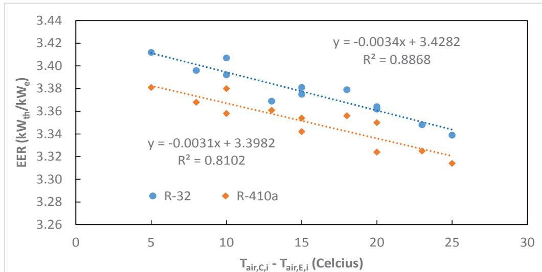
**Figure 14** Performance curves of R-32 and R-410a air-conditioners with 15 m of piping tube.
