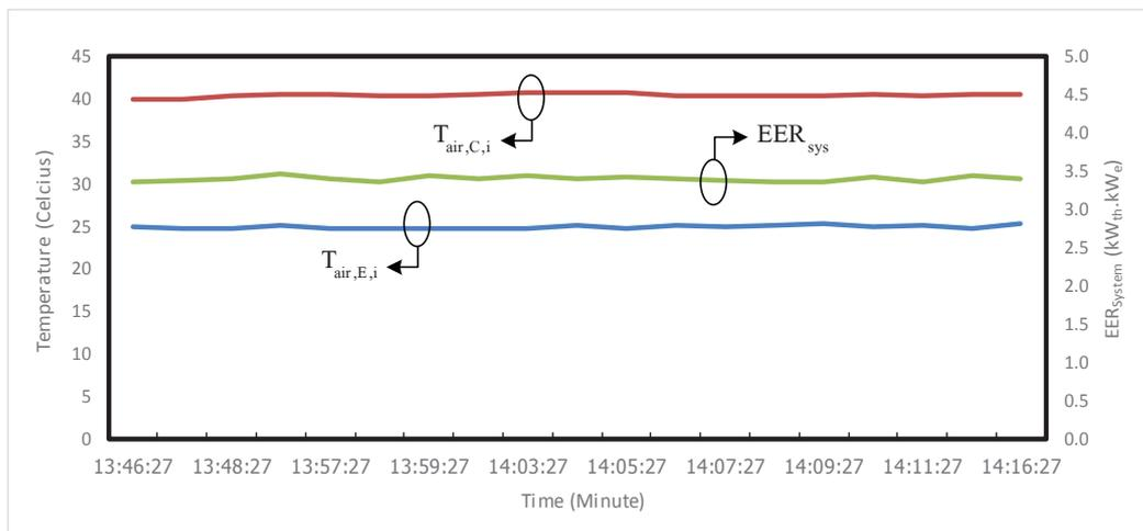
**Figure 12** The air temperature profile and  $EER_{sys}$  for R-410a air-conditioner at the air entering evaporator and condenser temperature around 25°C and 40°C with 10 m of piping tube.
