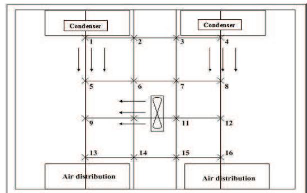
Figure 4 The measuring positions of the air temperature distribution in the condensing unit room.
