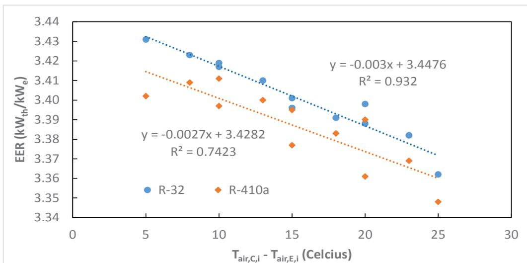
**Figure 13** Performance curves of R-32 and R-410a air-conditioners with 10 m of piping tube.
