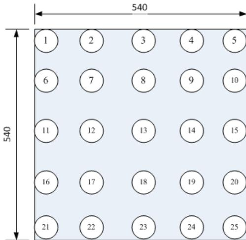
**Figure 5** The measuring positions of air velocity at the hood of the condenser.
