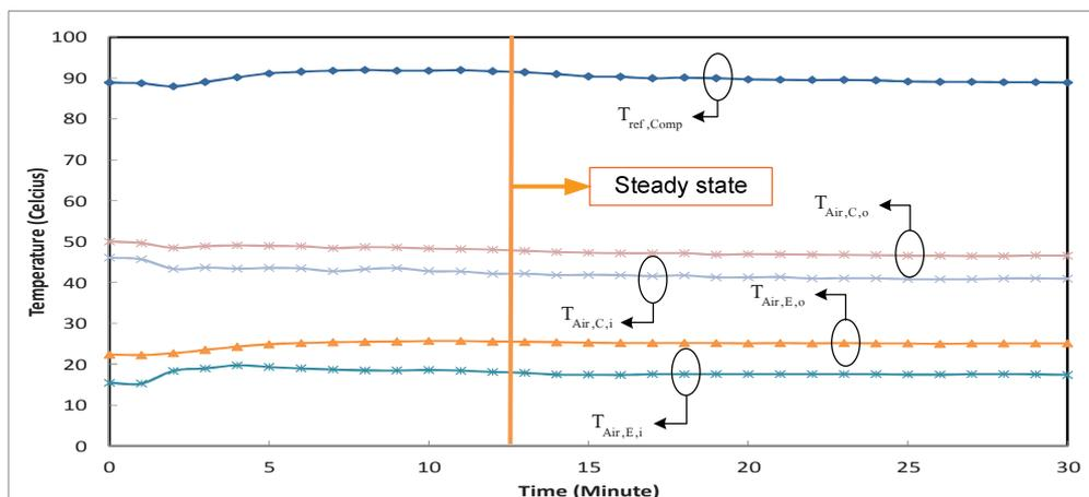
Figure 10 Temperature histories of the refrigerant and the room temperature for R-32 air-conditioner at the air entering evaporator and condenser temperature around 18°C and 40°C.
