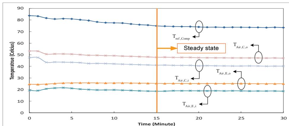
Figure 9 Temperature histories of refrigerant and room temperature for R-410a air-conditioner at the air entering evaporator and condenser temperature around 18°C and 40°C.
