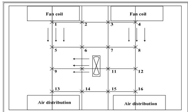
Figure 3 The measuring positions of the air temperature distribution in the evaporating unit room.
