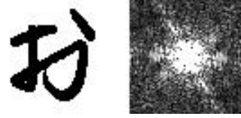
Fig.4: Input Pattern (Left, the Same Pattern in Fig. 1(a)) and Its Amplitude Fourier Spectrum Image (Right).
