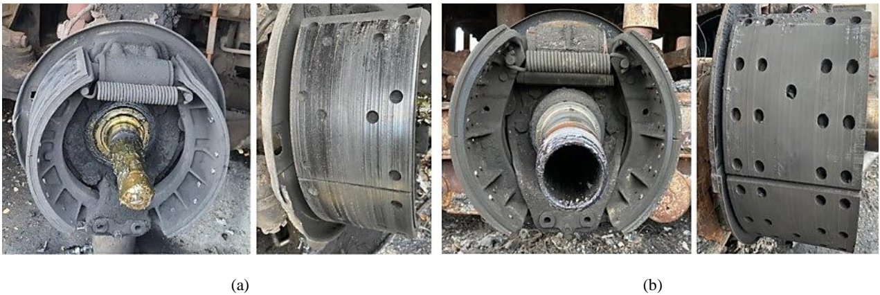
Figure 5 Air-over-hydraulic system: (a) front-axle wheel; (b) middle-axle wheel.
