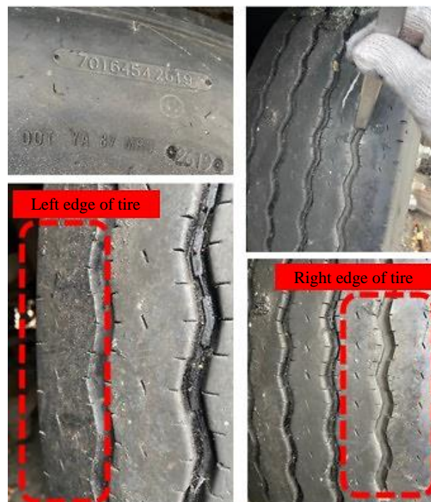
Figure 8 Tire condition of the front wheel of the bus.
