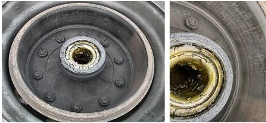
Figure 7 Small cracks on the drum brake surface at the front-axle wheel.
