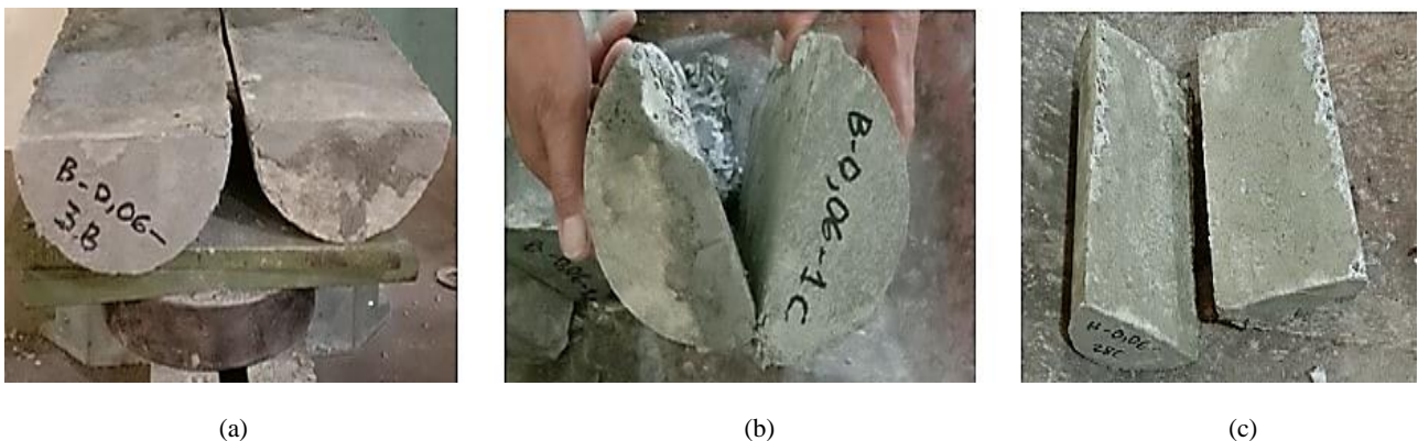
Figure 8 Tensile splitting test failure (a) mode A, (b) mode B, and (c) mode C
