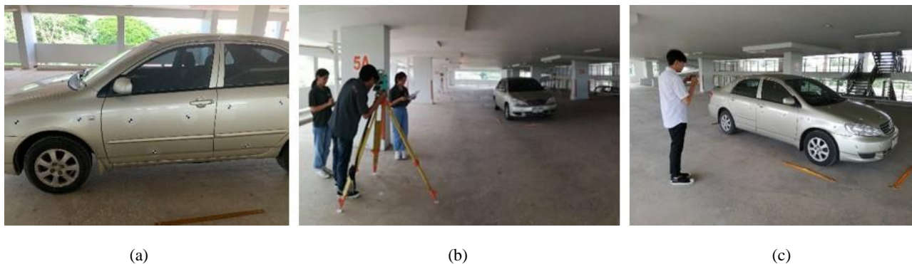
Figure 2 Data collection in this study: (a) targets established as control points and checkpoints; (b) total station survey for target locations; (c) example of image acquisition
