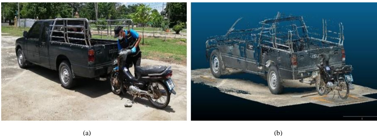
Figure 7 Comparison of the simulation for analyzing collision trajectory: (a) traditional forensic police method; (b) alignment of 3D models using the CloudCompare software
