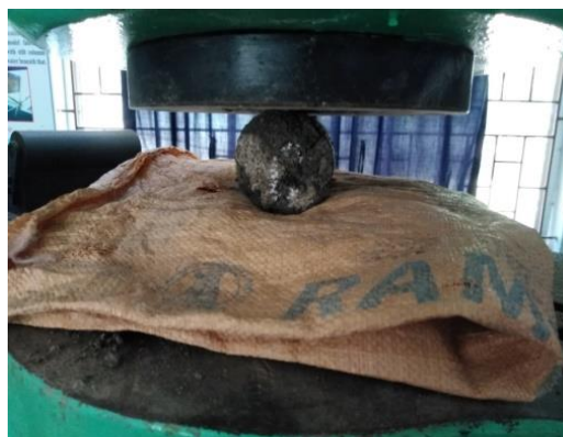
Figure 4 Testing of the cylinder for splitting tensile strength
