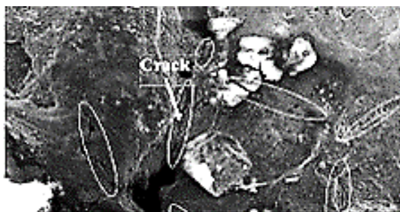
Figure 13 Micro-cracks on a workpiece surface at room temperature ( I = 7.5A ) ( \times 200 )
