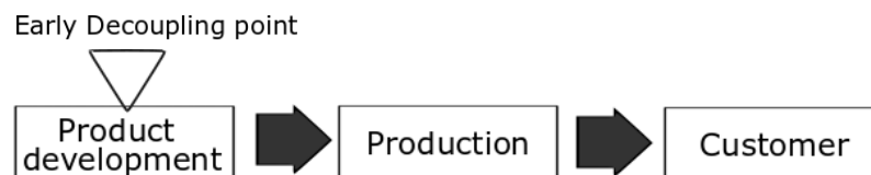
Figure 2. Shifting the decoupling point to an early stage through AM.
