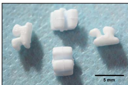
Figure 3. dental ceramic bracket fabricated by powder injection moulding.
