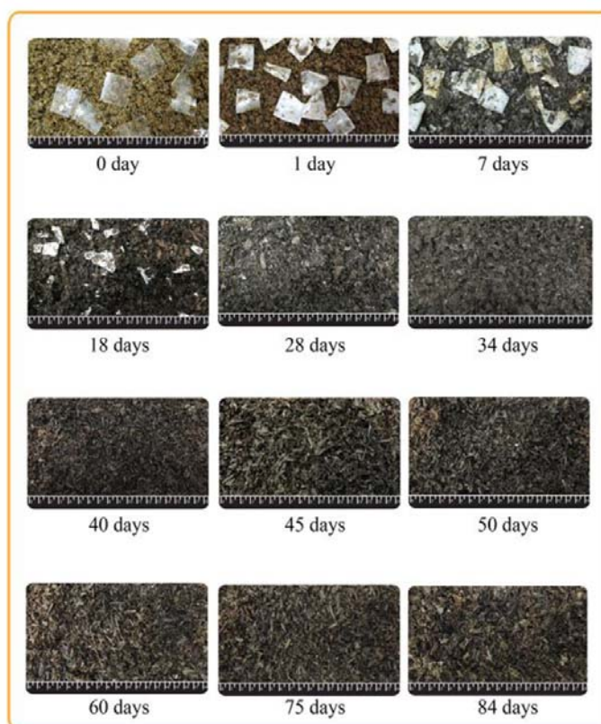
Figure 5. Appearance of the PLL film during the disintegration test. (Scale: 1 large division = 1 mm, 1 small division = 0.5 mm).
