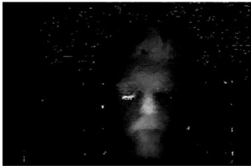
Figure 4. Generated disparity map by SGM method.
