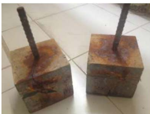
Figure 15. The sample of concrete crack.
