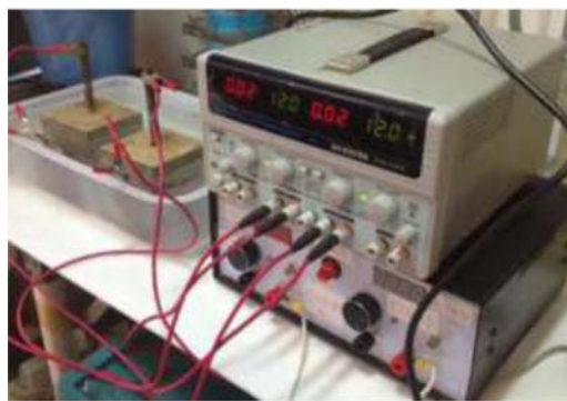
Figure 7. The accelerated corrosion test.
