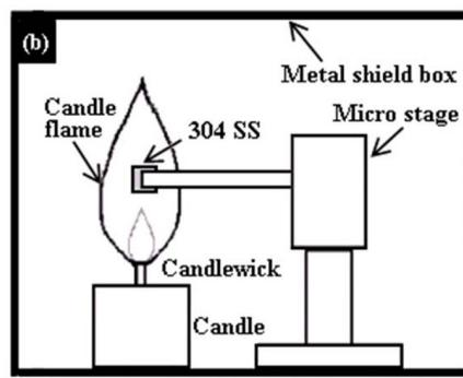
**Figure 1.** (a) Temperature distribution of candle flame. (b) Schematic of an experimental setup for combustion synthesis of CLCNOs.
