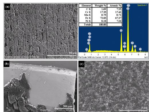
**Figure 2.** SEM analysis: (a) SEM image and EDX spectra of 304 SS before experiment, (b) and (c) SEM images of CNMs on 304 SS substrate at ×60 and ×10,000 magnifications, respectively.
