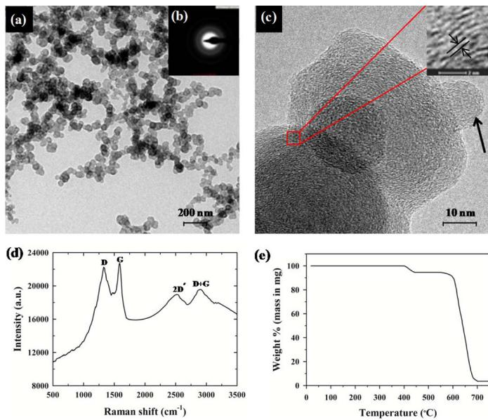
**Figure 3.** Morphology and characteristics of CLCNOs: (a) TEM image, (b) SAED pattern, (c) High-magnification TEM image, (d) Raman spectra and (e) The thermal stability of the CLCNOs from TGA analyze.
