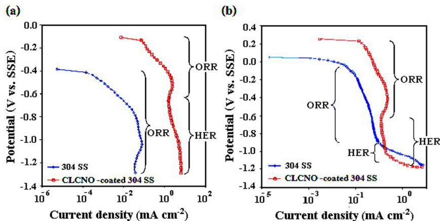
**Figure 5.** Cathodic polarization behavior of CLCNO-coated stainless steel compared with 304 SS cathodes: (a) in KOH solution and (b) in  $\text{H}_3\text{PO}_4$  solution.
