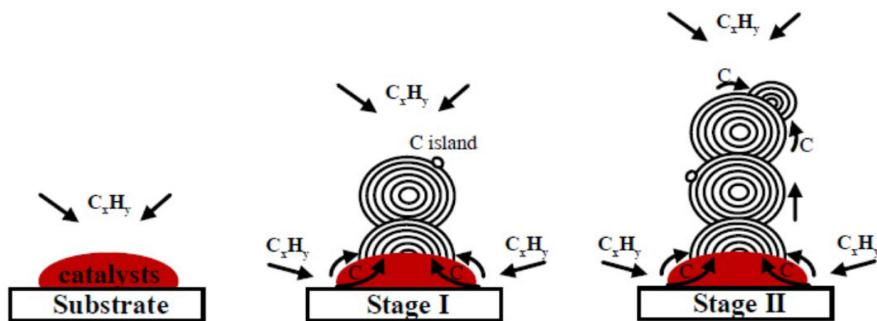
**Figure 4.** Schematic diagram for describing the growth mechanisms of CLCNOs on 304 SS.
