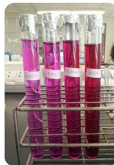
Figure 2. A photograph of various concentrations of cresol red solution (pH 9.0) from 0.001 to 0.008 % (w/v) (left to right).
