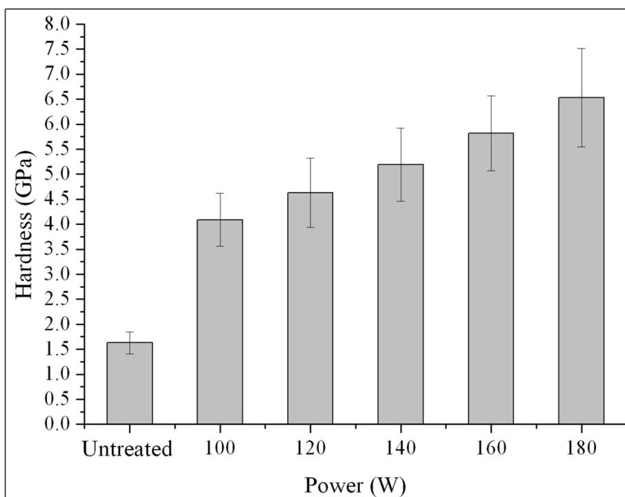
**Figure 8.** Hardness of uncoated titanium and the titanium coated at 100, 120, 140, 160 and 180 W.
