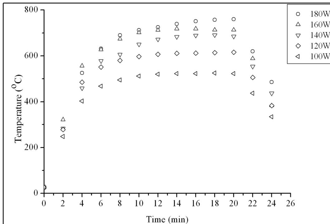
**Figure 2.** Temperature as a function of processing time for the titanium coated at 100, 120, 140, 160 and 180 W.
