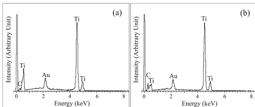
**Figure 4.** EDS spectra for titanium coated at (a) 100 W and (b) 140 W.
