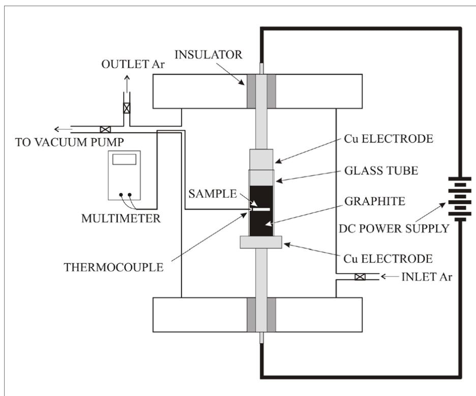
**Figure 1.** Schematic diagram of the apparatus used for coating process.
