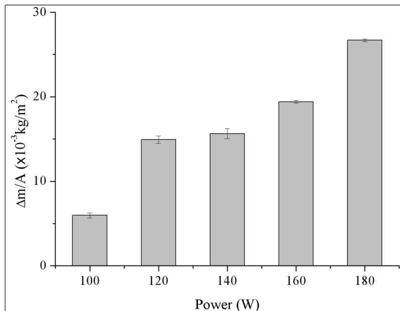
**Figure 3.** Mass change of coated titanium as a function of applied electric power.
