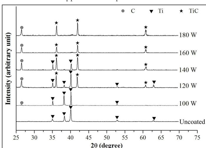
**Figure 6.** XRD patterns for uncoated titanium and the titanium coated at 100, 120, 140, 160 and 180 W.
