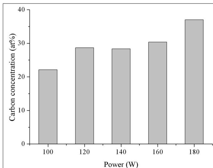
**Figure 5.** Concentration of carbon in the coated titanium as a function of applied electric power.
