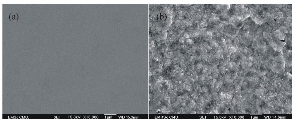
**Figure 7.** SEM micrographs for uncoated titanium and the titanium coated at 120 W.
