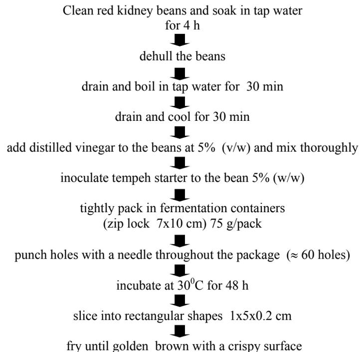
**Figure 2. Process of red kidney bean tempeh production** (adapted from Chompreeda [6]).
