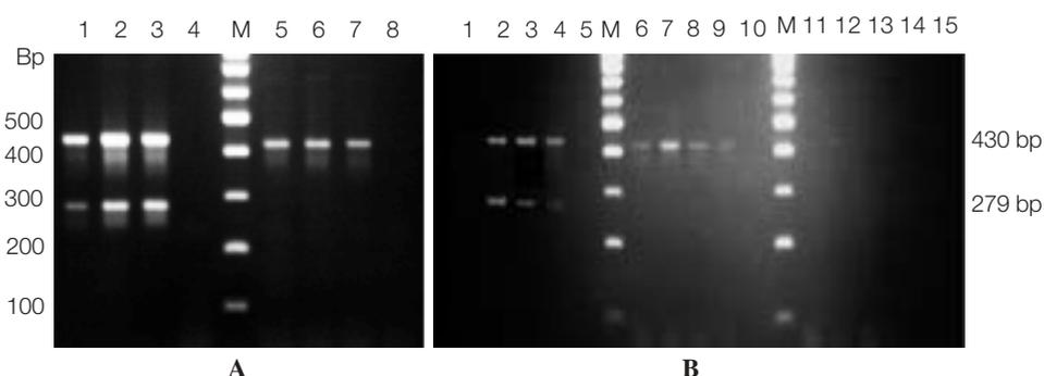
Fig 3—Agarose gel-electrophoresis of PCR products using two sets of primers obtained with various concentrations of primers (A) and with different annealing temperatures (B) for pathogenic *Leptospira* pyrogenes and non-pathogenic *Leptospira* patoc.
