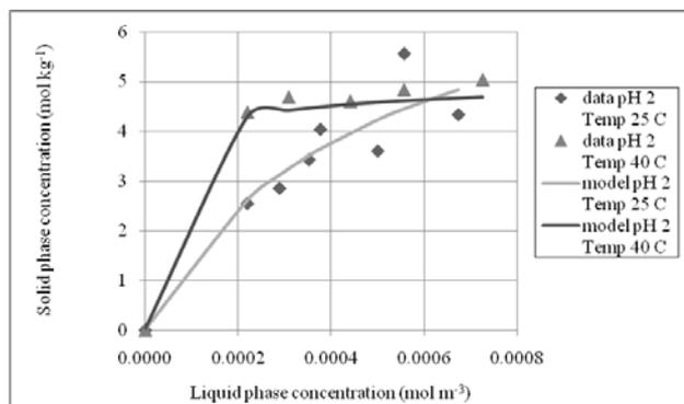
**Figure 3.** Lactic acid removal from liquid phase by Amberlite IRA-96 for pH2 at temperature 25 °C and 40°C.
