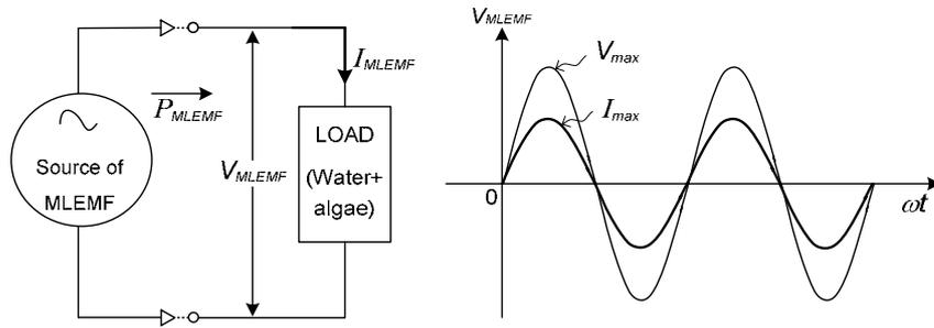
**Figure 4** Output signal of voltage of MLEMF system
