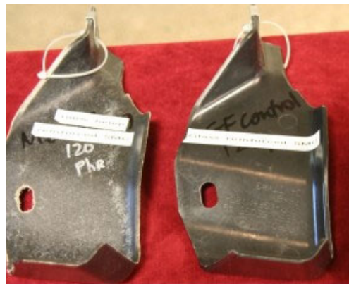
Figure 3 Part of hemp and glass reinforced plastic bonded with resin solutions for bus seat [7]
