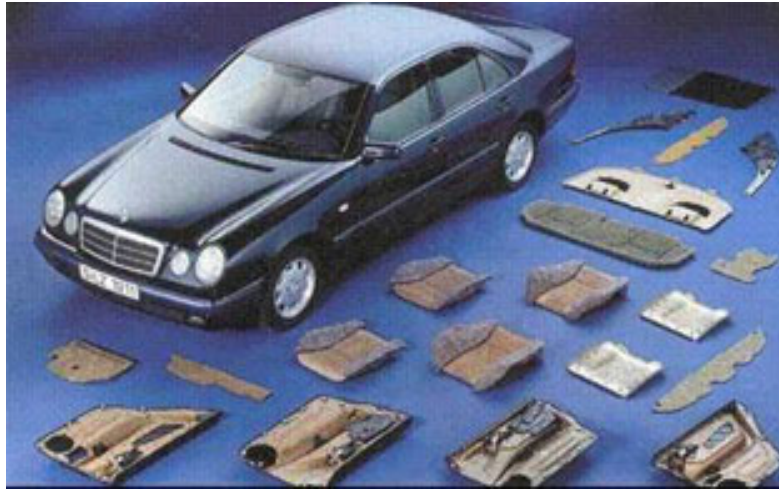
Figure 5 Interior components made of natural fiber composite for E Class car [9]
