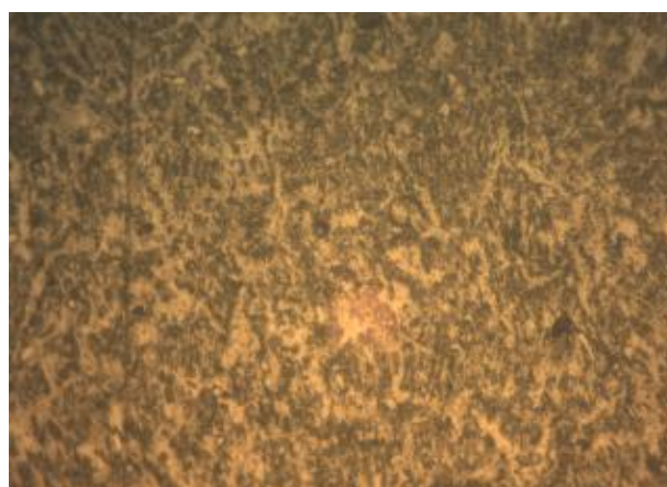
Plate 3. Microstructure of China weldment (X 400) (Authors' Estimate, 2008).
