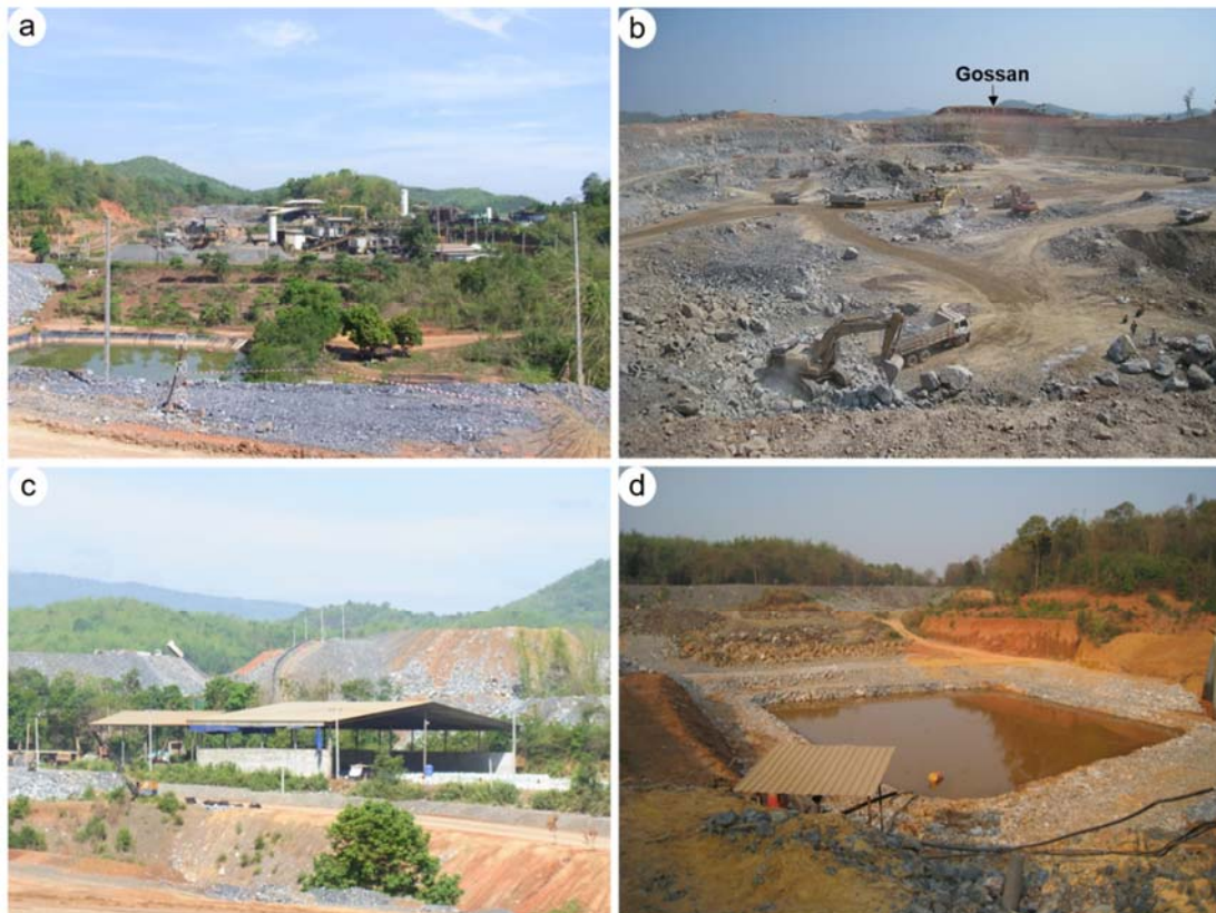
Figure 1 Photographs of mining activities in the study area such as (a) gold processing plant, (b) mining pit showing location of dumped waste rocks of ore-barren gossan in (c, d) the dump sites.
