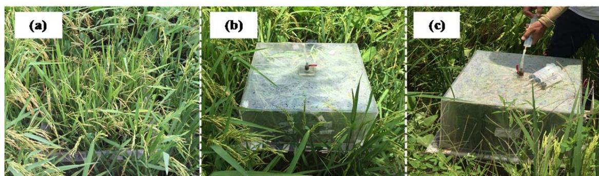
**Figure 2** (a) rice plantation in rice field; (b) collecting gas in the chamber; and (c) gas sampling
