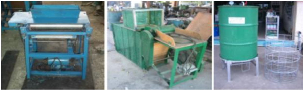
Figure 1 Fibre crushing machine, carding machine and boiler
