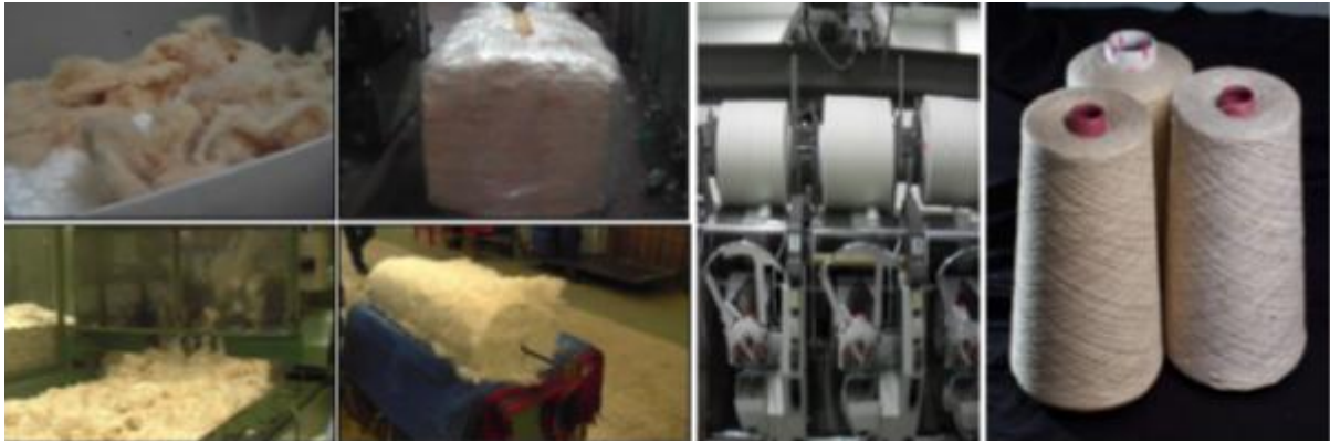
Figure 3 Mixing and producing fibre laps in the open- end spinning process
