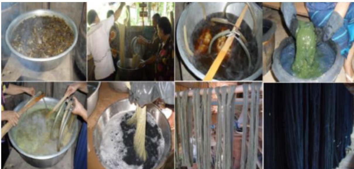
Figure 4 Colour dyeing of palm fibre yarns: green from Indian almond ( Terminalia catappa ) leaves and blue from the indigo plant
