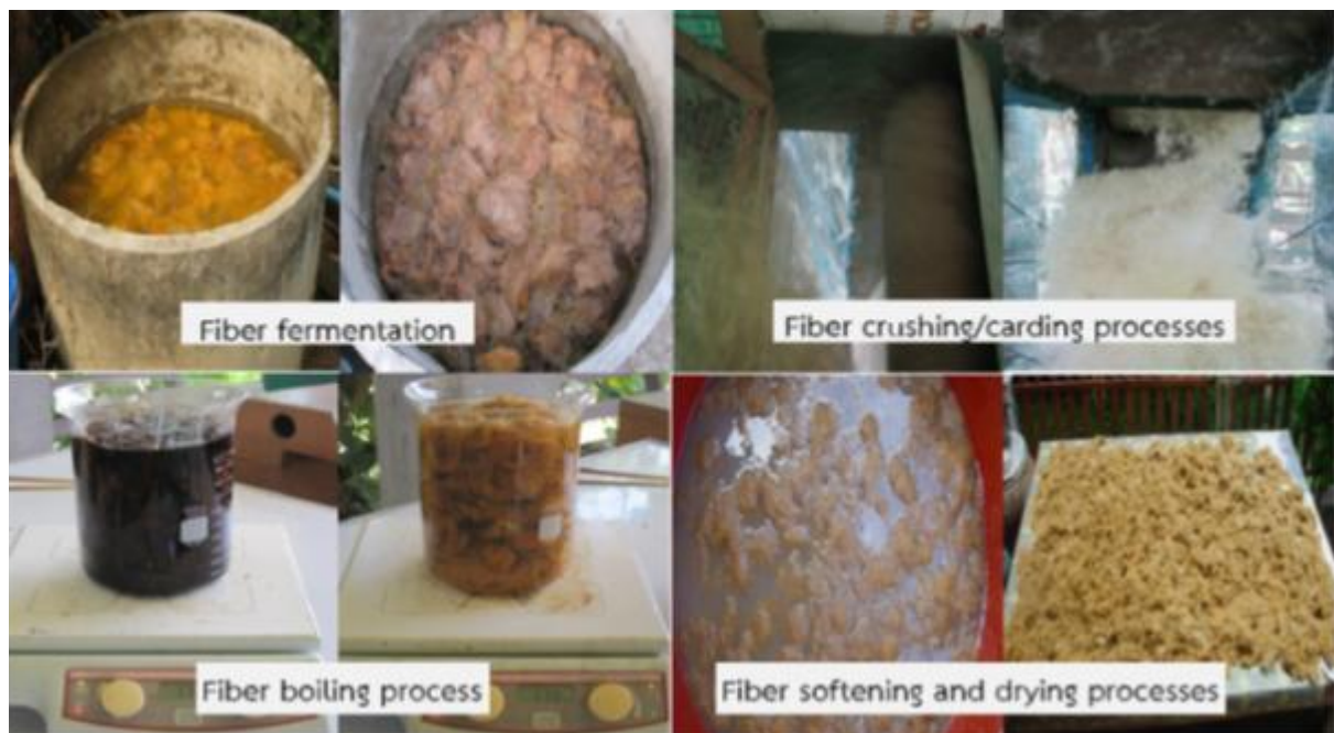
Figure 2 Improvement of palm fibre through fermentation under anaerobic conditions followed by physical processing (boiling, crushing and carding)
