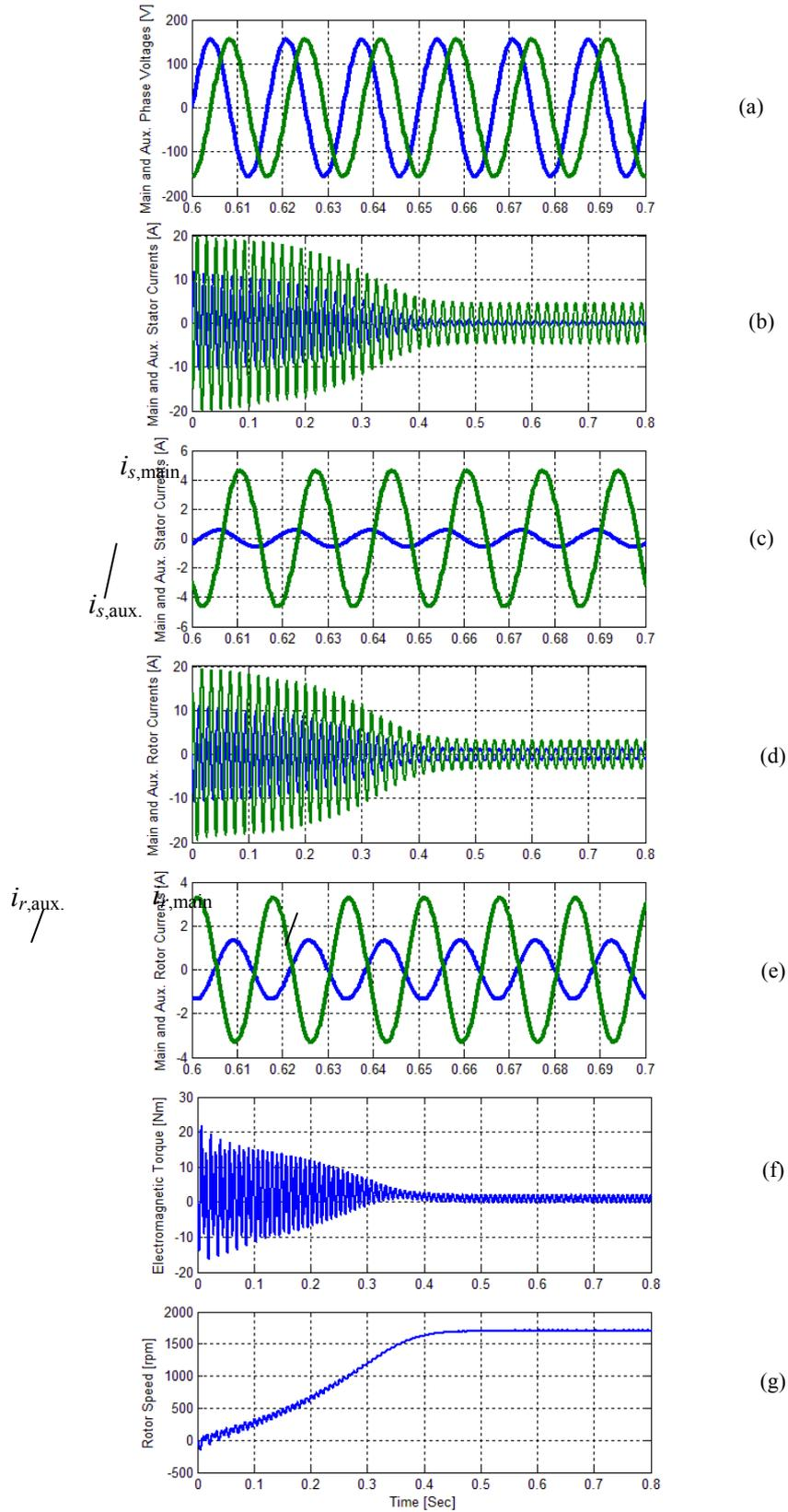
**Figure 10. Simulation results of the main and auxiliary two-phase induction motor ( $v_{main} = v_{aux.} = 110 V_{rms}$ ) at full-load condition.**
