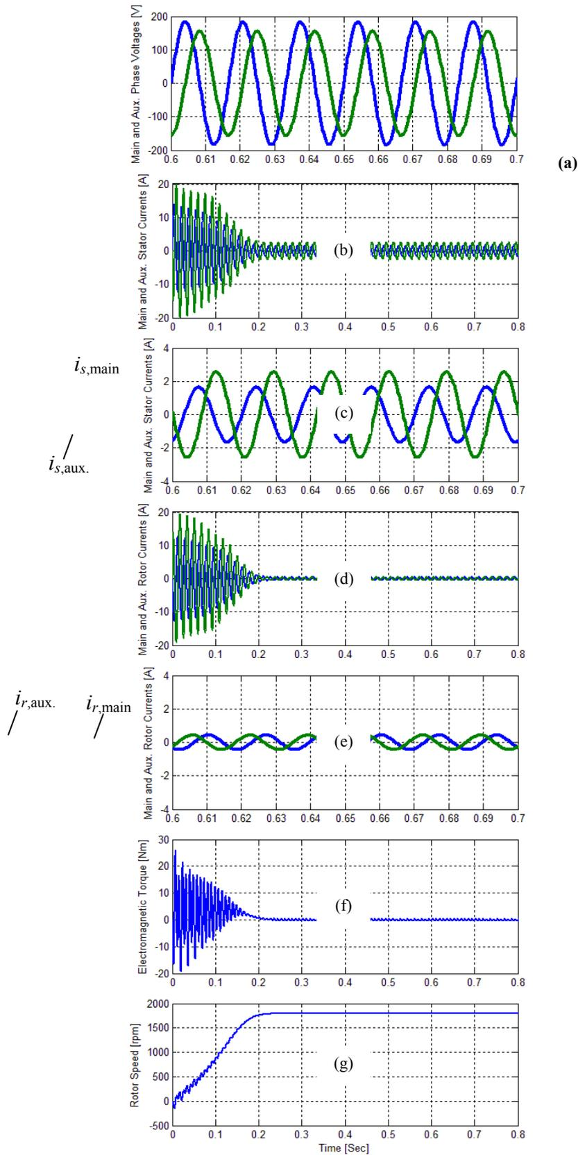
**Figure 7. Simulation results of the main and auxiliary two-phase induction motor ( $v_{\text{main}} = 110V_{\text{rms}}$  and  $v_{\text{aux.}} = a*110V_{\text{rms}}$ ) at no-load condition.**
