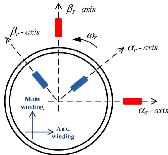
**Figure 1. Asymmetrical two-phase induction motor.**
