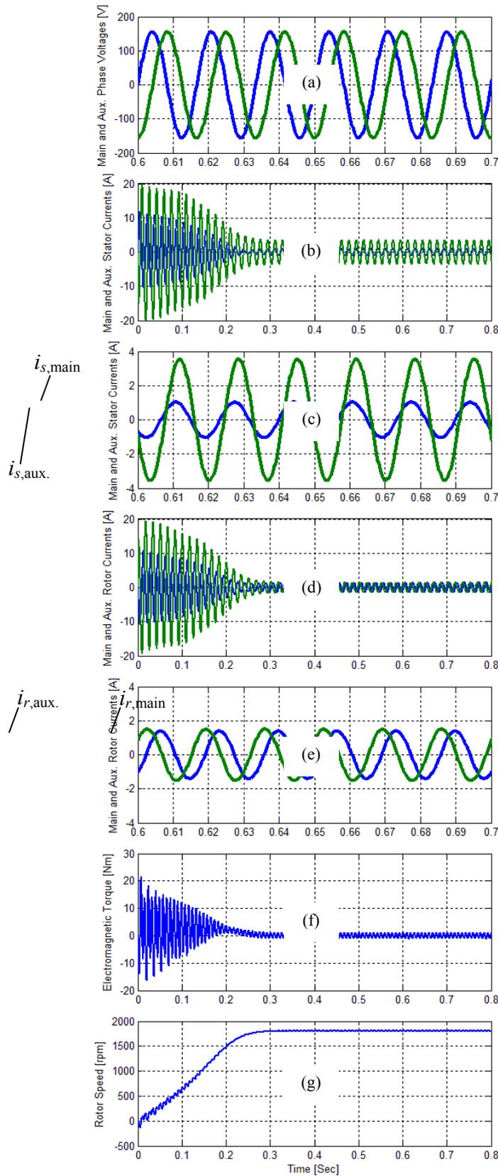
**Figure 8. Simulation results of the main and auxiliary two-phase induction motor ( $v_{\text{main}} = v_{\text{aux.}} = 110 \text{ V}_{\text{rms}}$ ) at no-load condition.**
