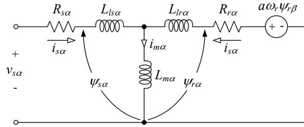
(a) Auxiliary winding in  $\alpha$  - axis.
