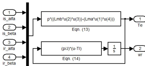
Figure 5. Electromagnetic torque and rotor speed equations.
