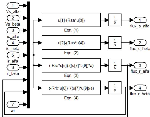
Figure 3. Stator and rotor voltage equations.
