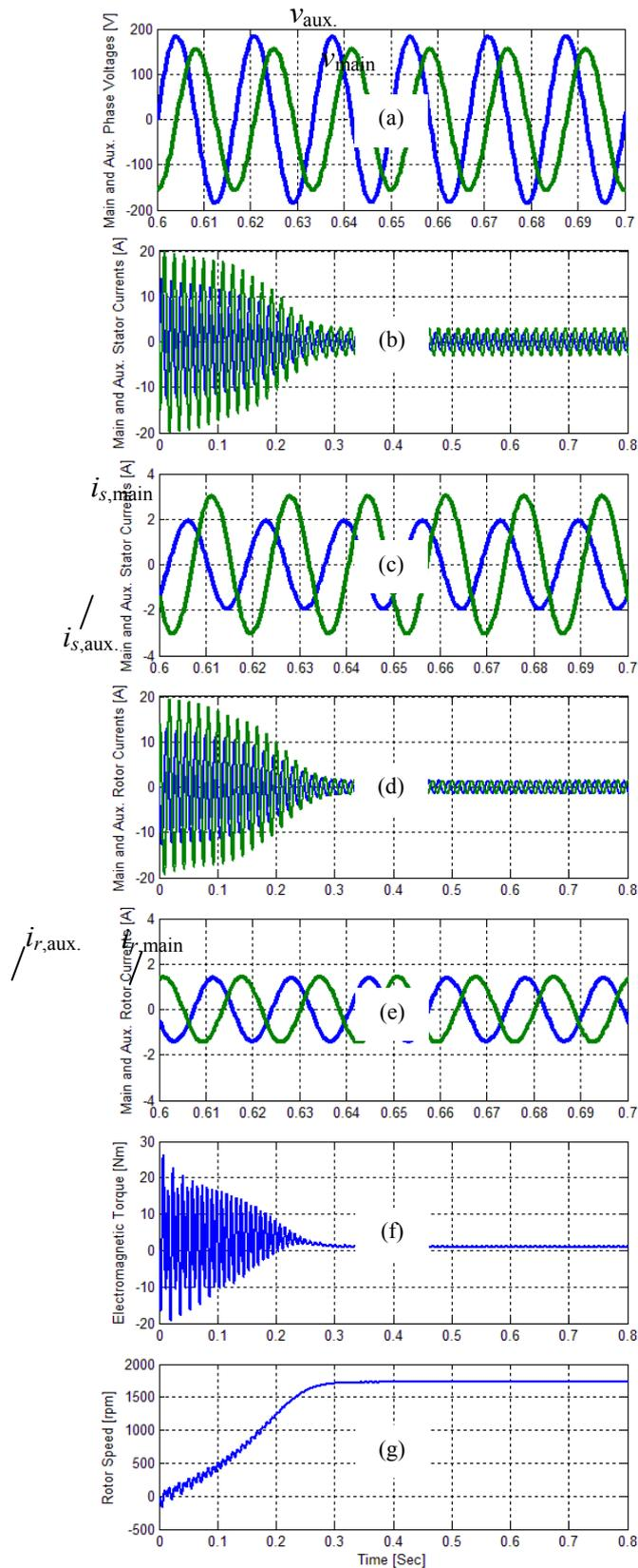
**Figure 9. Simulation results of the main and auxiliary two-phase induction motor ( $v_{main} = 110V_{rms}$  and  $v_{aux.} = a*110V_{rms}$ ) at full-load condition.**
