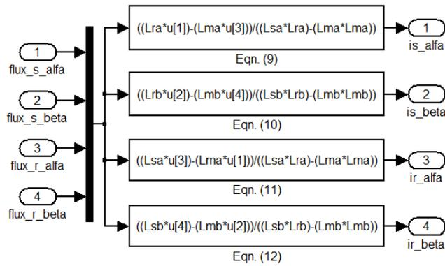
Figure 4. Stator and rotor current equations.
