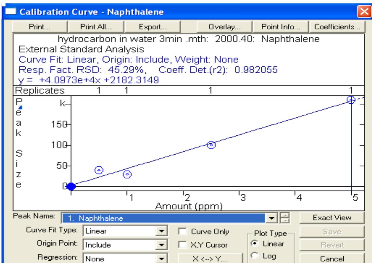
Figure 2. Standard Calibration Curve of Naphthalene.
