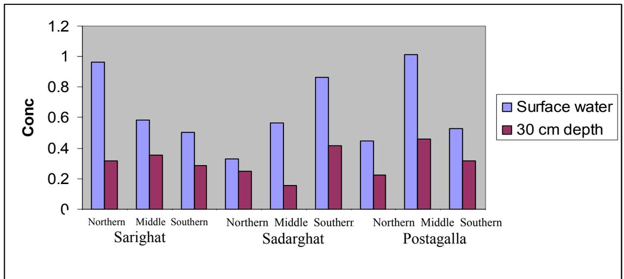
**Figure 4. Concentrations of naphthalene in surface and 30 cm depth of water at the northern, middle and southern side of Sowarighat, Sadarghat and Postagolla sampling stations of the Buriganga River.**
