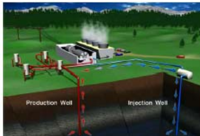
Fig.1 Schematic of geothermal power plant
