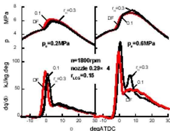
Fig. 8 Effects of LCG addition on combustion process under low and high engine loading.
