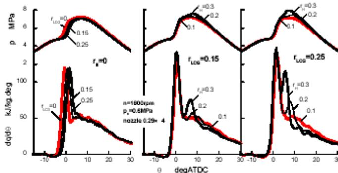
**Fig. 6** Effects of LCG addition on combustion process at high engine load of  $p_e=0.6\text{MPa}$ .
