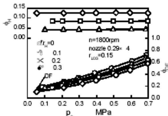
**Fig. 10** Combustion efficiency of hydrogen against engine load.
