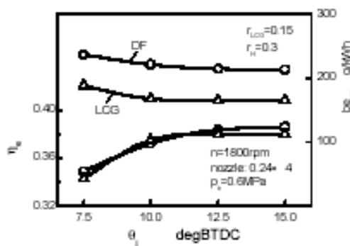
Fig. 12 LCG behavior under various injection timing.
