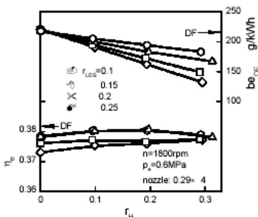
Fig. 4 Effects of LCG addition on engine performance at fixed engine load.
