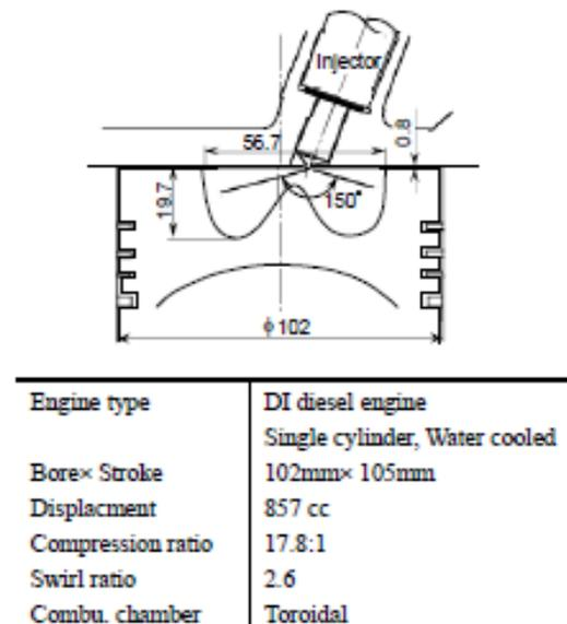
Fig. 1 Engine specification.
