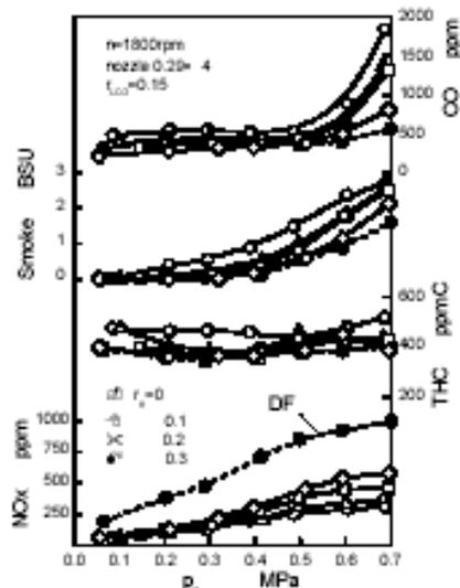
Fig. 11 Effects of LCG composition on emissions under various engine loading.
