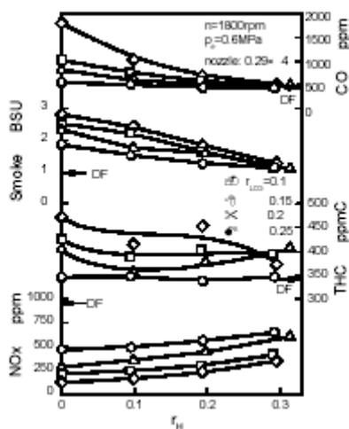
Fig. 5 Effects of LCG addition on emission at high engine load of  $p_e=0.6$  MPa.
