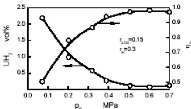
Fig. 9 Combustion efficiency of hydrogen against engine load.
