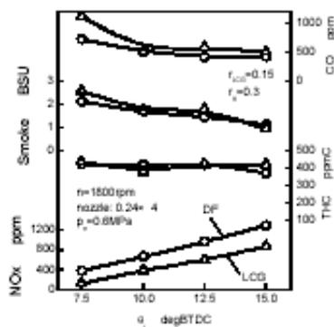
Fig. 13 LCG behavior under various injection timing.
