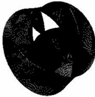
Fig. 4 Hybrid grid of rotor zone.
