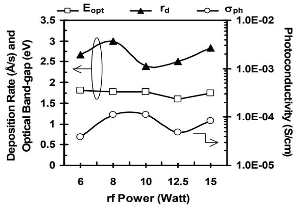
**Figure 2.** The characteristics of i-layers which resulted under optimization of rf power.
