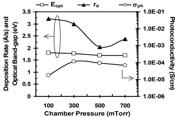
**Figure 3.** The characteristics of i-layers which resulted under optimization of chamber pressure.
