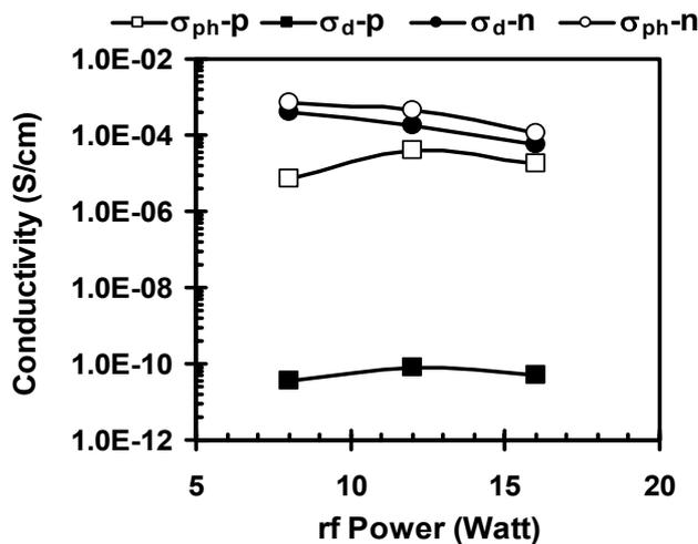
**Figure 4.** Conductivity of p- and n-layers under optimization of rf power.
