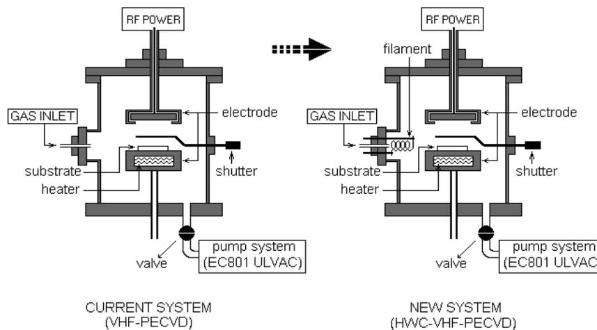
**Figure 1.** The home made VHF-PECVD reactor system: current system and new system.
