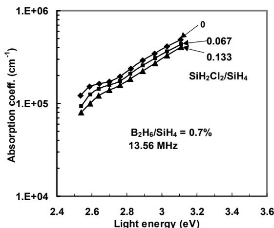
**Figure 2.** Change of absorption coefficient by small amount of  $\text{SiH}_2\text{Cl}_2$  for p( $\mu\text{c-Si}$ ) made from conventional gas mixture ( $\text{SiH}_4 + \text{B}_2\text{H}_6 + \text{H}_2$ )
