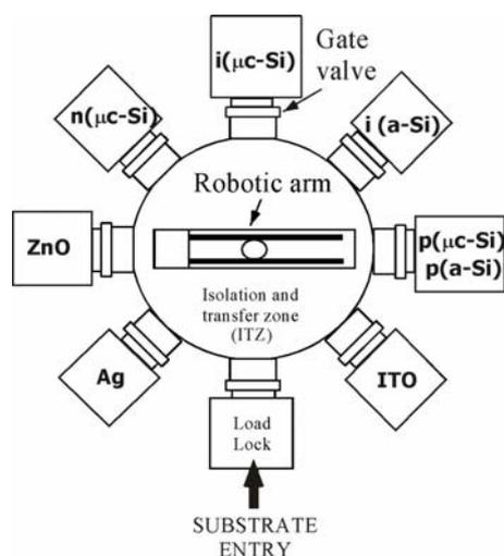
**Figure 1.** Chamber layout of the system used for cell fabrication.
